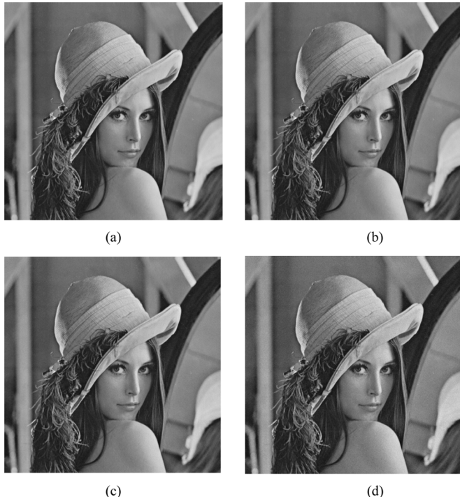
Fig. 5. Cover image and stego images under various payloads. (a) Cover image. (b) Stego image, 2 bpp at 46.86 dB. (c) Stego image, 3 bpp at 40.97 dB. (d) Stego image, 4 bpp at 34.90 dB.
